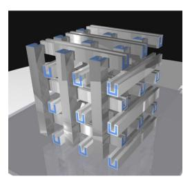
Fig.1: Artist's view of a 3D photonic metamaterial composed of elongated split-ring resonators made by DLW of a polymeric backbone (blue) and subsequent coating via metal CVD.
